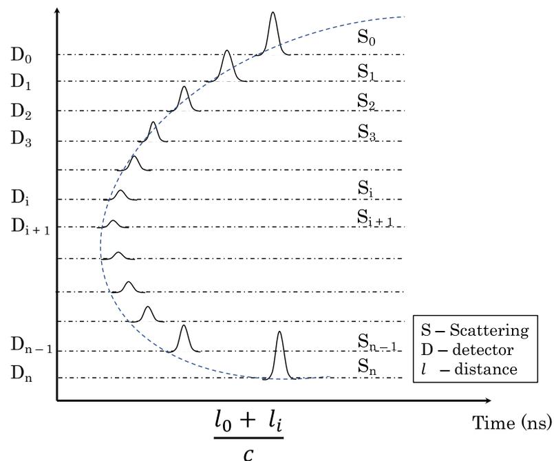
**Figure 3.** Principle of the proposed time gate to identify the pollutant particles from the correct scattering center. Due to the pulsed emission of the incident laser source, scattering from different scattering centers will arrive at the detector at different time intervals  $t_i = \frac{l_0+l_i}{c}$  where  $l_0$  is the known distance from the laser to the scattering particle source and  $l_i$  is the distance from the scattering particle to the  $i$ th detector.
