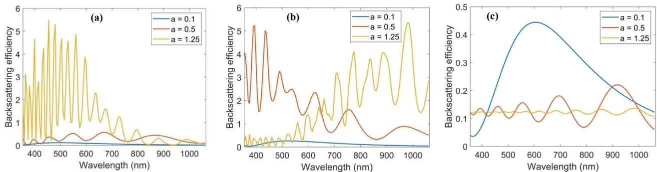
**Figure 5.** Back scattering intensity from (a) pure water, (b) contaminated water and (c) black carbon as a function of the wavelength of the incident laser for various particle radii  $a = 0.1 \mu\text{m}$ ,  $0.5 \mu\text{m}$ , and  $1.25 \mu\text{m}$ .
