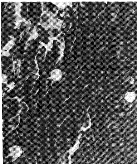
Fig. 4 Typical inclusion identified as manganosilicate containing sulphur
