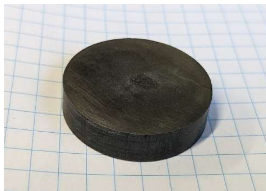
Figure 3.7: A section of a sample produced by spark-plasma sintering.
