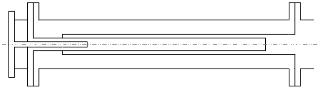
Fig. 2.9 Triple tube for preheating zone.
