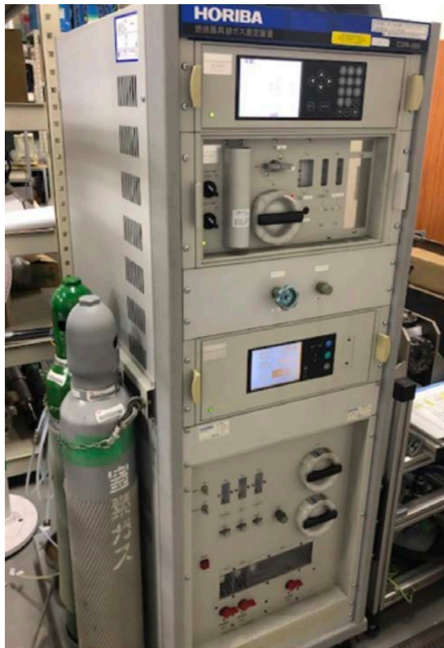
Fig. 2.19 Photograph of the gas analyzer (COPA-3000) .
