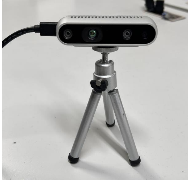
Figure 10 Realsense D435i used in this experiment.
