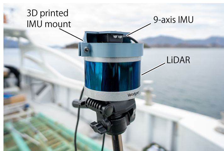
Figure 4.11 Sensor configuration of LiDAR and IMU
