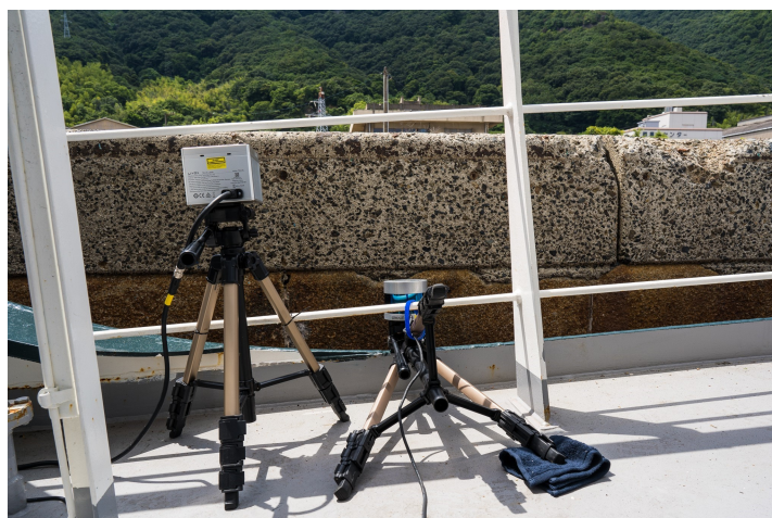
Figure 4.28 LiDAR (on left) for berth line detection.
