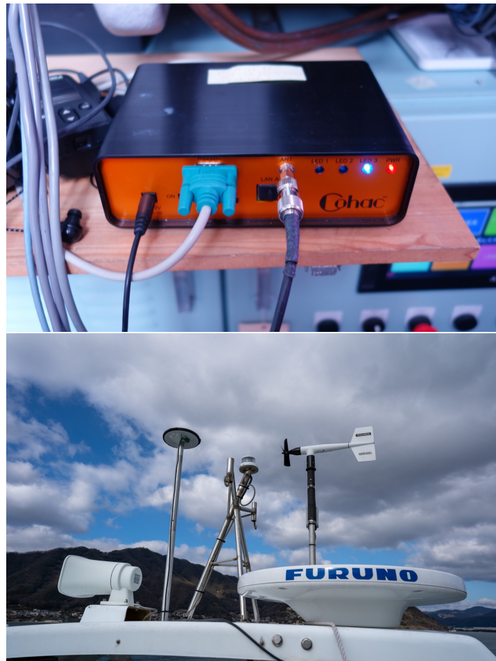
Figure 3.13 Sensors installed on "Shinpo". QZSS Receiver (TOP), Anemometer, GPS compass, antenna for QZSS (LOW)
