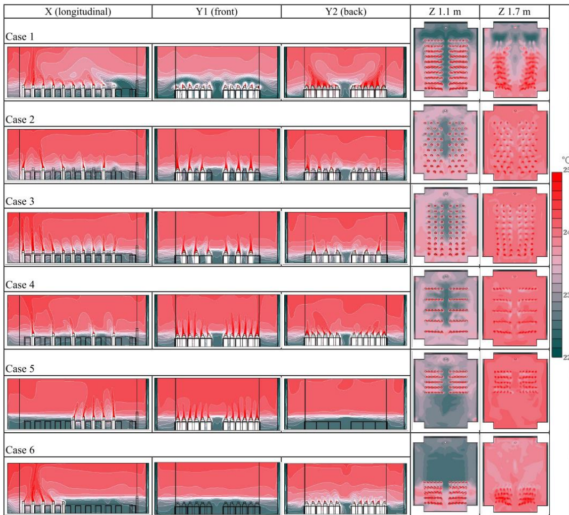
Figure 2.7 Temperature contours for different seating patterns cases
