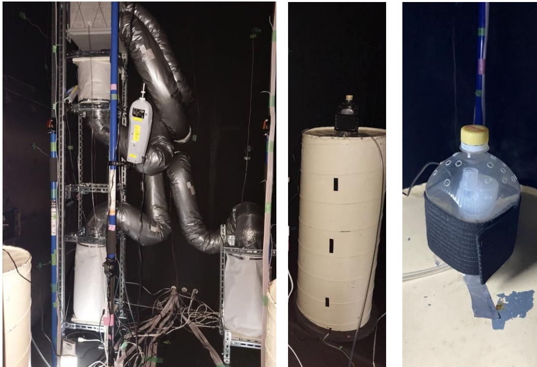
a. PDV unit and DV diffuser
