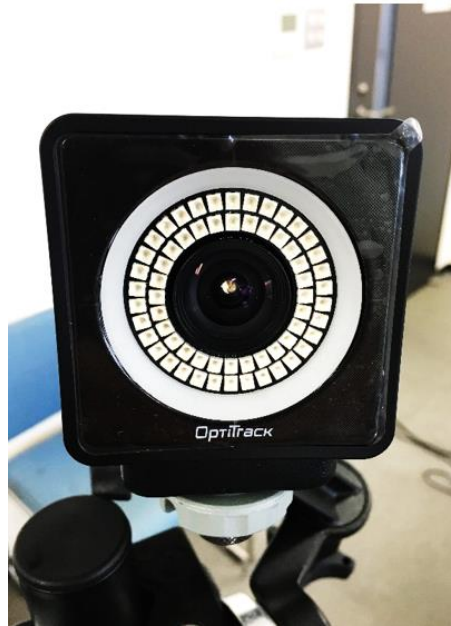
Figure 5. 3 A high-speed camera in the optical tracking system
