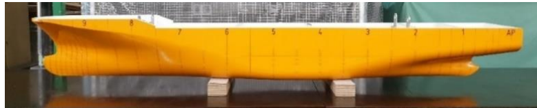
FIGURE 2.2: RIOS containership model at Osaka University Towing tank facility
