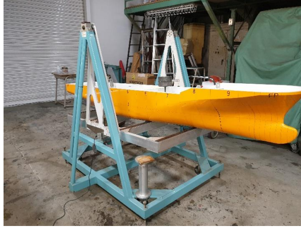
FIGURE 2.3: Adjustment of the Radius of Gyration
