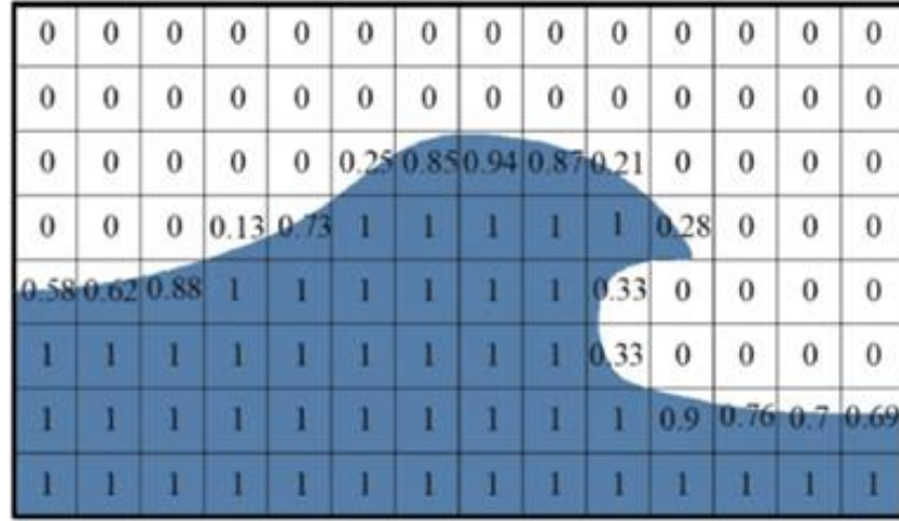
Figure 3.5. The volume fraction of fluid in each grid cell (Nguyen-Thi et al., 2021)
