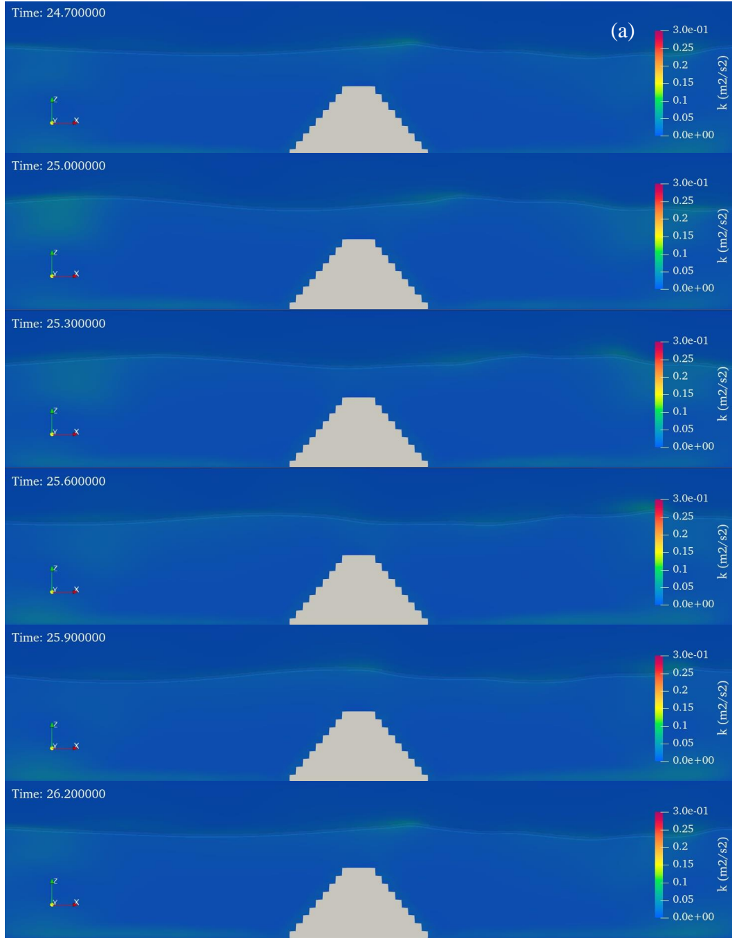
Figure B.2a. The evolution of turbulent kinetic energy over a micro rough slope breakwater ( S_h=0.06\text{m} ) in case of B=0.25\text{m}
