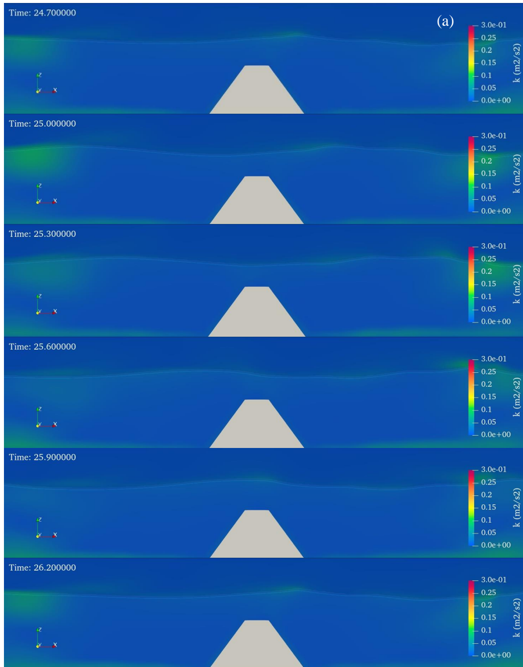
Figure B.1a. The evolution of turbulent kinetic energy over a smooth slope breakwater ( S_h=0\text{m} ) in case of B=0.25\text{m}
