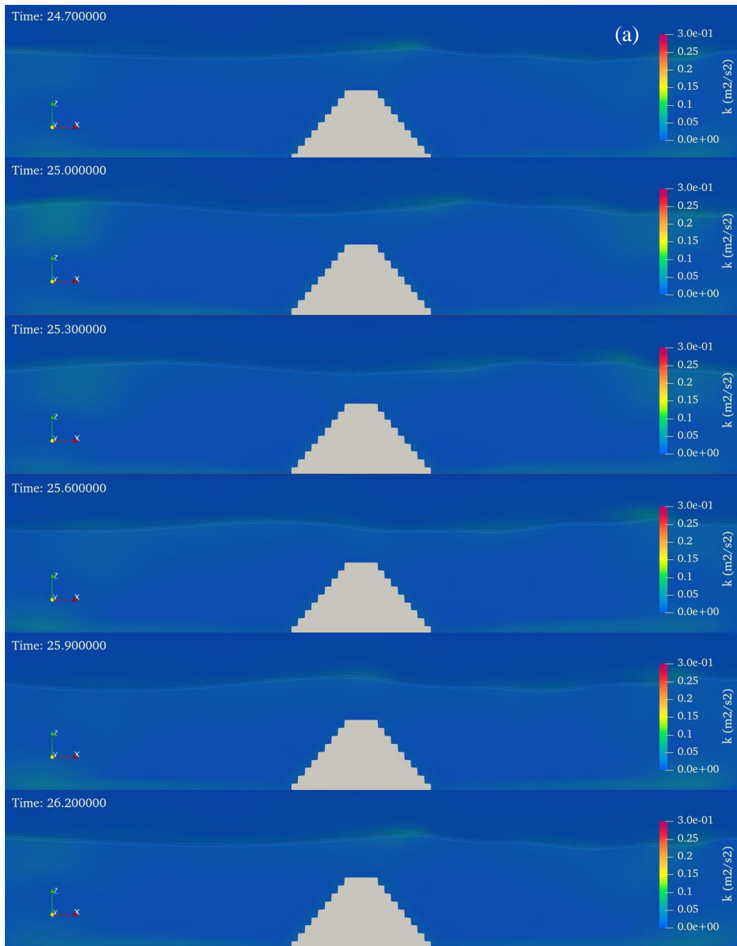
Figure B.2a. The evolution of turbulent kinetic energy over a micro rough slope breakwater ( S_h=0.06m ) in case of B=0.25m
