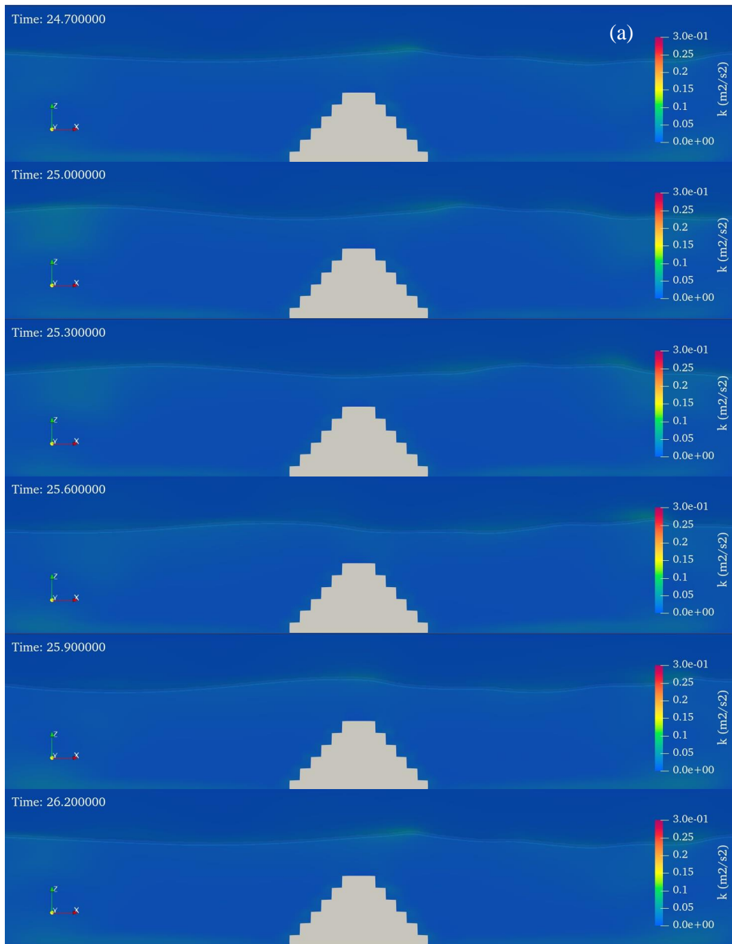
Figure B.3a. The evolution of turbulent kinetic energy over a macro rough slope breakwater ( S_h=0.09\text{m} ) in case of B=0.25\text{m}
