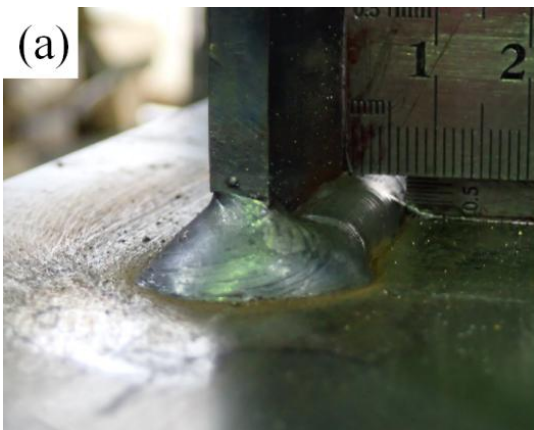
Fig.1.7 Appearance of weld toe. (a) As-welded toe, and (b) HFMI-treated toe.
