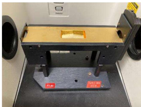
Figure 4-2-1. Photograph of the specular reflectance accessory (FT-80, Spectra-tech) with a wire-grid polarizer attached to a spectrometer.
