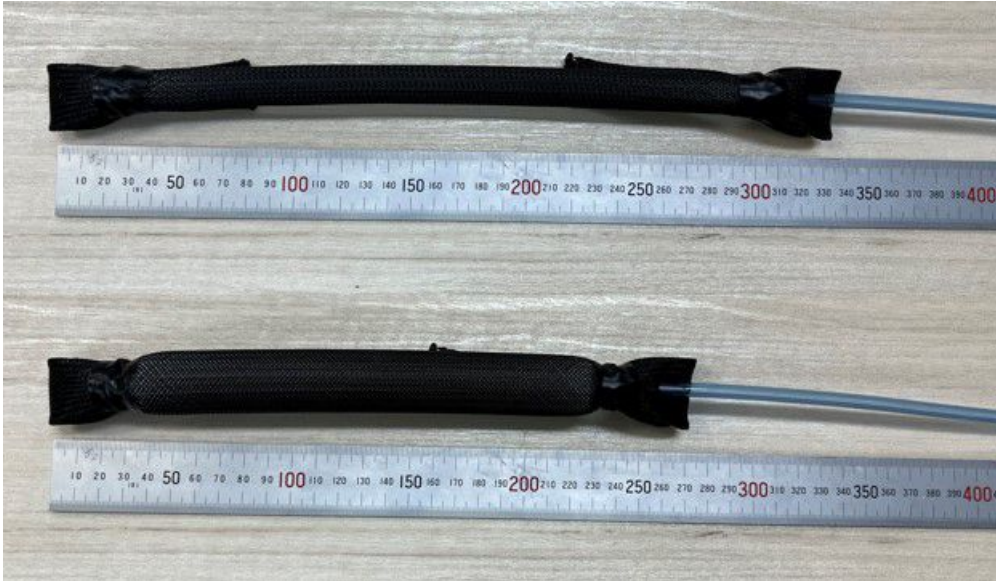
Figure 3.7: Natural state (top) and air-supplied state (bottom) of McKibben-type pneumatic artificial muscle
