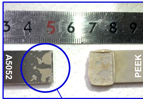
Interfacial delamination + Extensive PEEK cohesive breakdown
