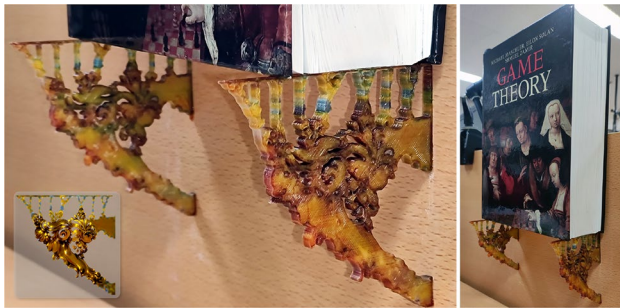
Fig. 17 3D-printing results of stylized topological optimized structures. The prompt was “golden, Baroque style”. The stylized structures were 3D-printed using the XYZ da Vinci Color mini
