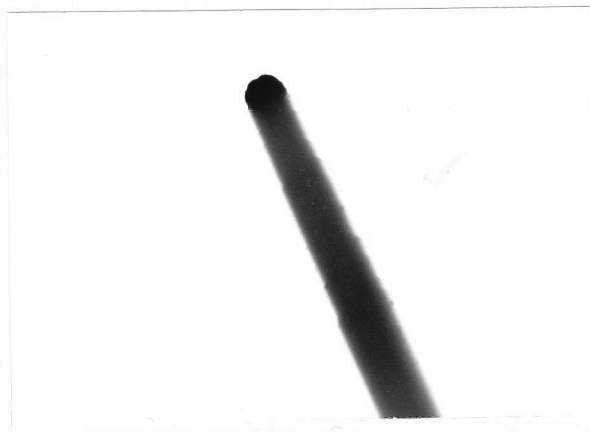
Fig.29 TEM photo. of a normal form silicon whisker with steeped shape grown at 950°C.
