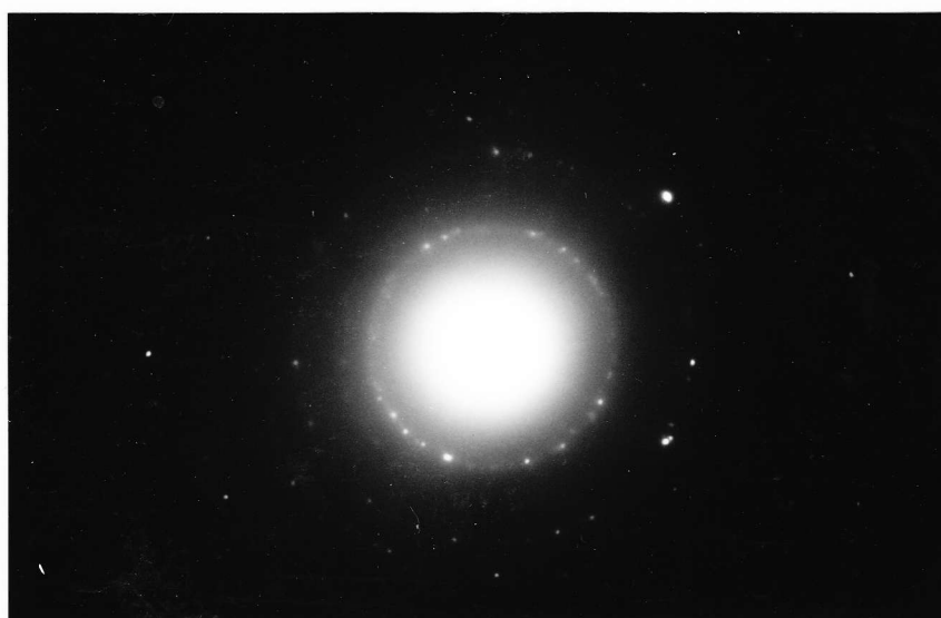
Fig.14 TED pattern of an annealed whisker after the crust is etched off. Note that unidentified rings disappear.
