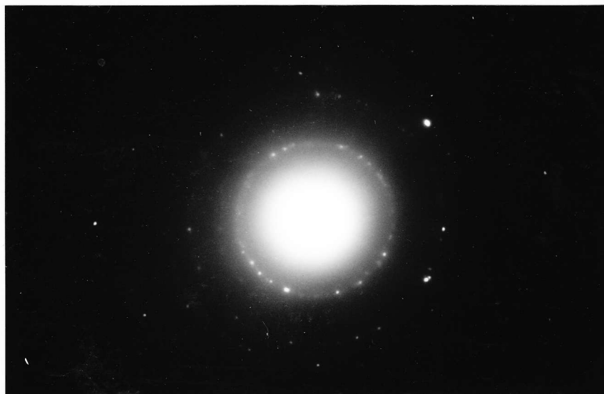
Fig.14 TED pattern of an annealed whisker after the crust is etched off. Note that unidentified rings disappear.
