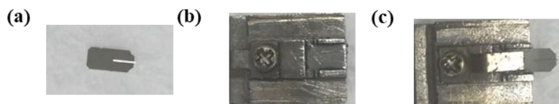
Figure 3.8 (a) Cantilever, (b) cantilever holder and (c) a fixed cantilever to the holder.
