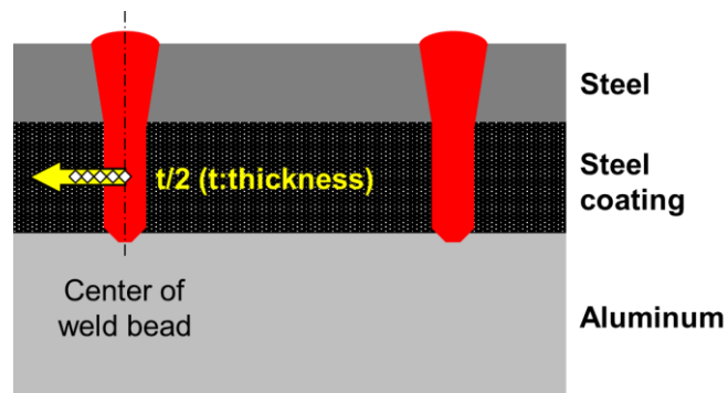
Fig. 5.8 Schematic illustration of hardness measurement.
