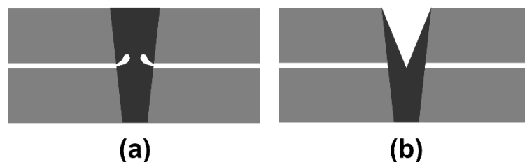
Fig. 1.9 Representative welding defects: (a) porosity, (b) underfill.
