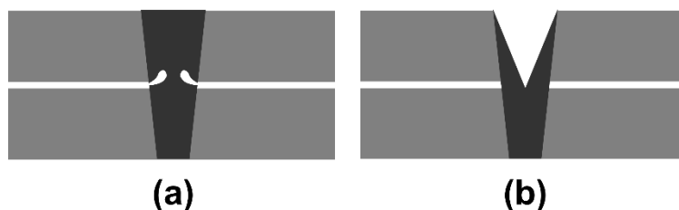
Fig. 1.9 Representative welding defects: (a) porosity, (b) underfill.
