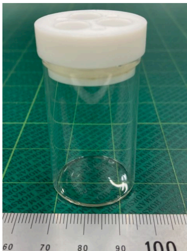
Fig. 3-6. Cell for chrono-coulometry.
