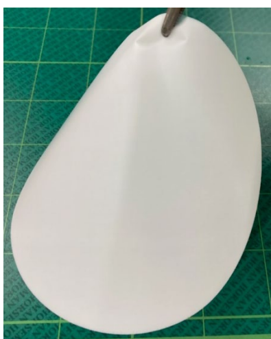
Fig. 4-11. Porous membrane used for the electrochemical impedance spectroscopy of the symmetric system.
