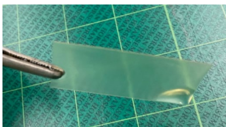
Fig. 3-14. Cation exchange membrane used for the discharge test.
