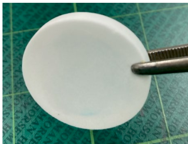
Fig. 3-3. Glass filter installed in the H-shaped cell.
