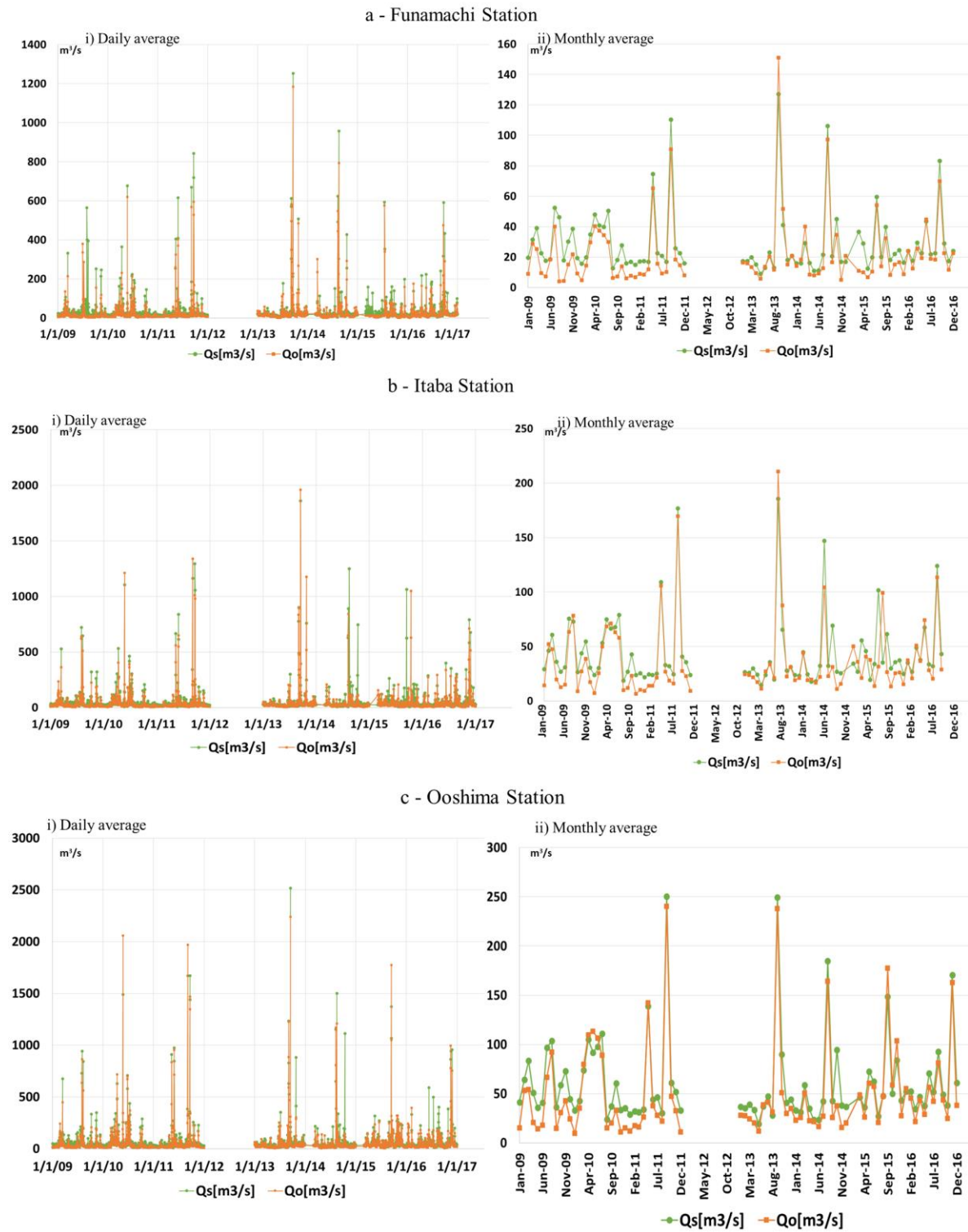
Fig. 29 - Daily and monthly averages for observed (orange) and simulated (green) values of discharged freshwater in the three monitoring stations of the Kako River
