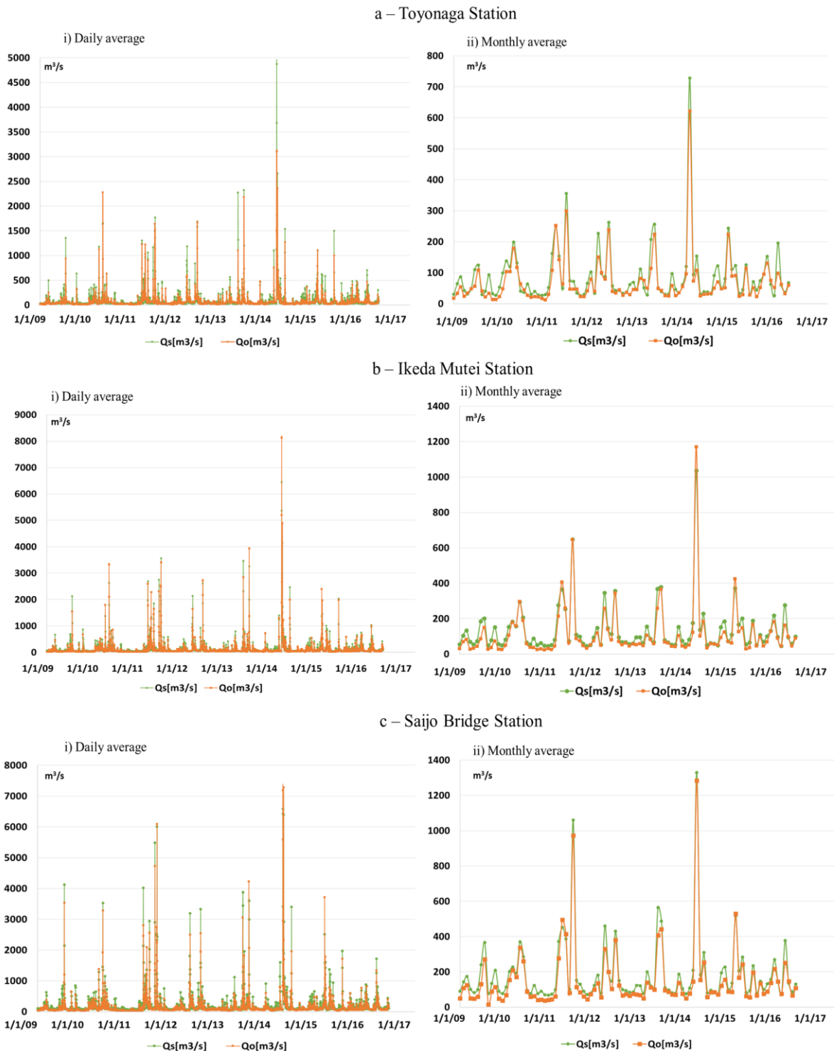
Fig. 30 - Daily and monthly averages for observed (orange) and simulated (green) values of discharged freshwater in the three monitoring stations of the Yoshino River
