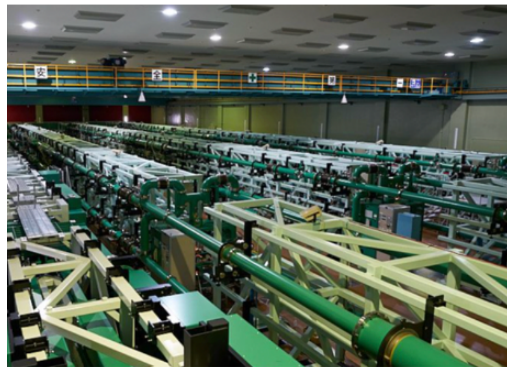
Figure 2.5. Laser amplifier of GEKKO-XII.
