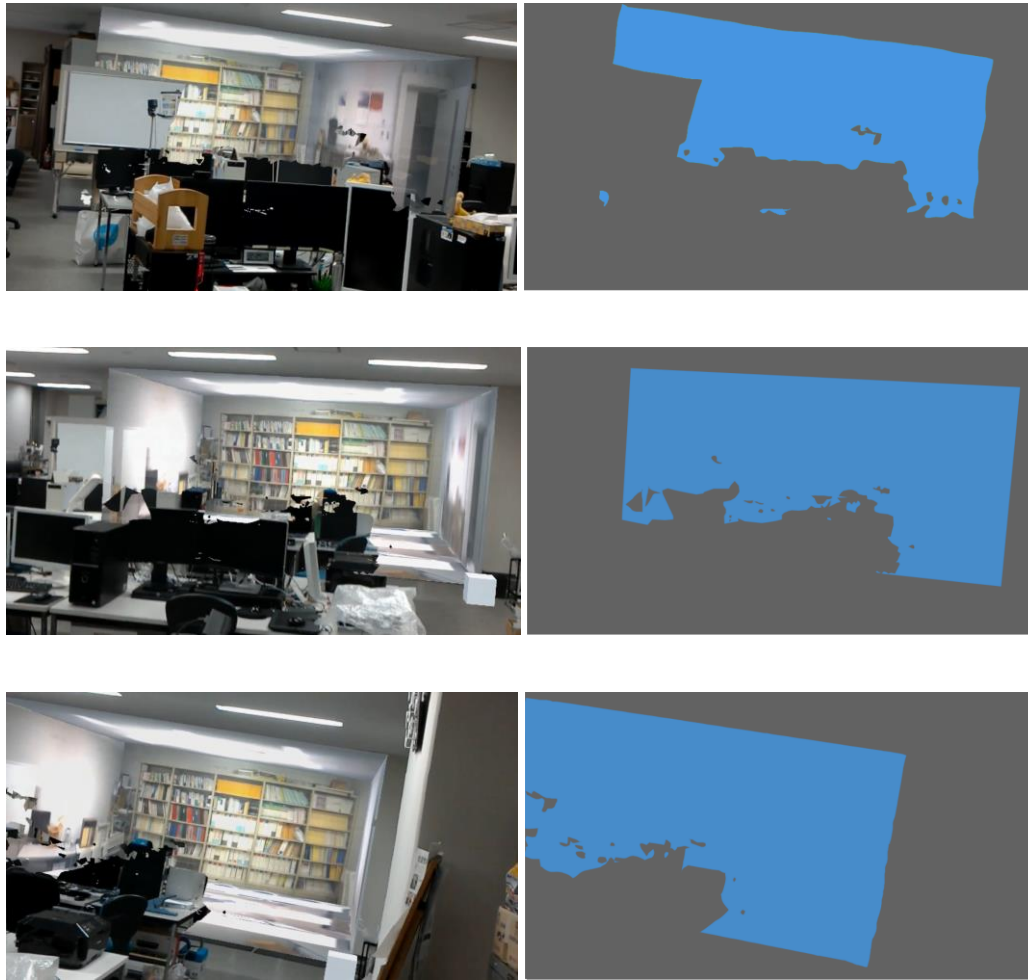
Figure 4.16. DR result and its segmentation map in position A (Above), B (Middle), C (Bottom) (Blue area as the mask region)
