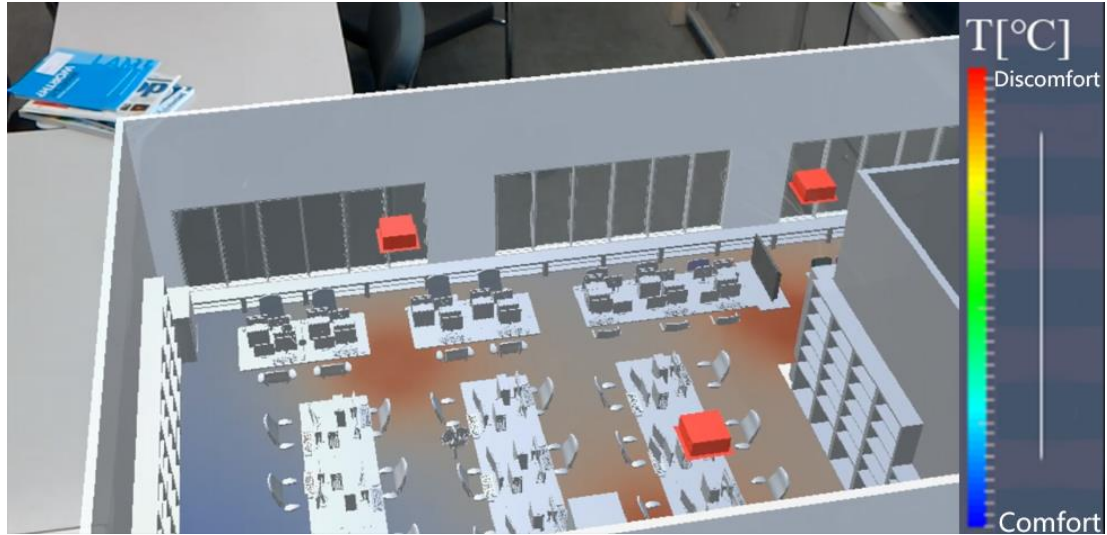
Figure 3.16. Heat map of room 411 small-scale model (1/10)
