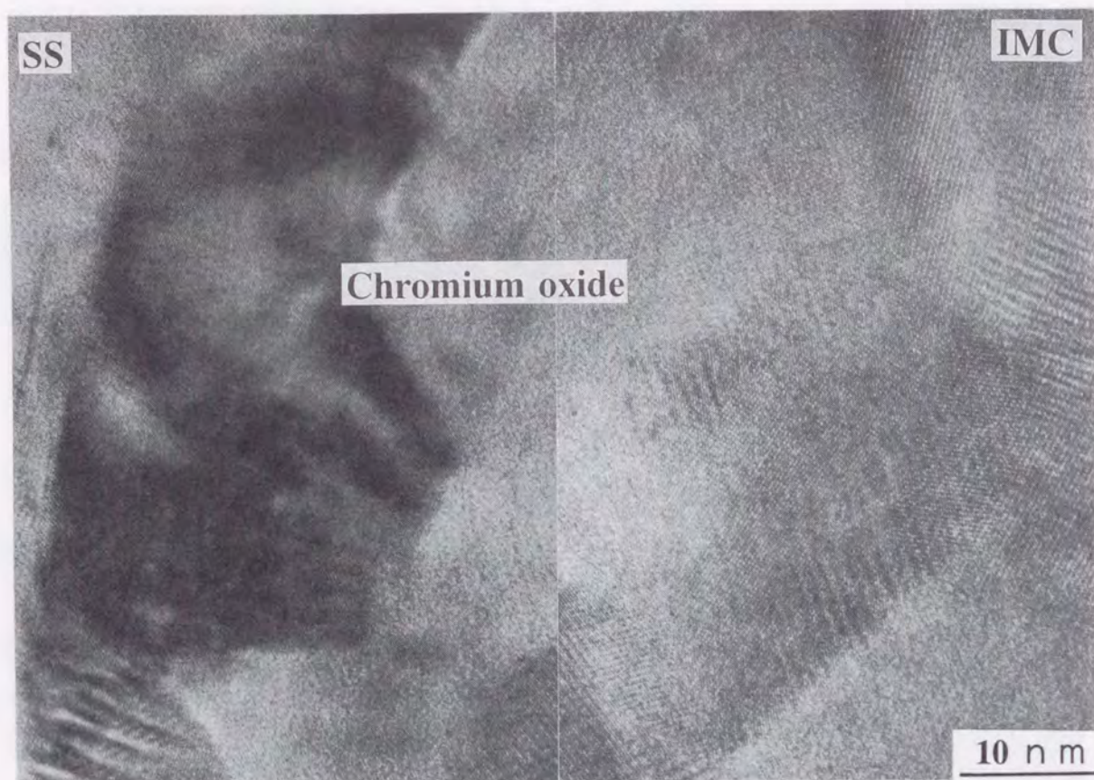
Fig. 3.13 TEM micrograph of chromium oxide layer around intermetallic compound (IMC) at interface of SS/A1 roll bonding sheet.
