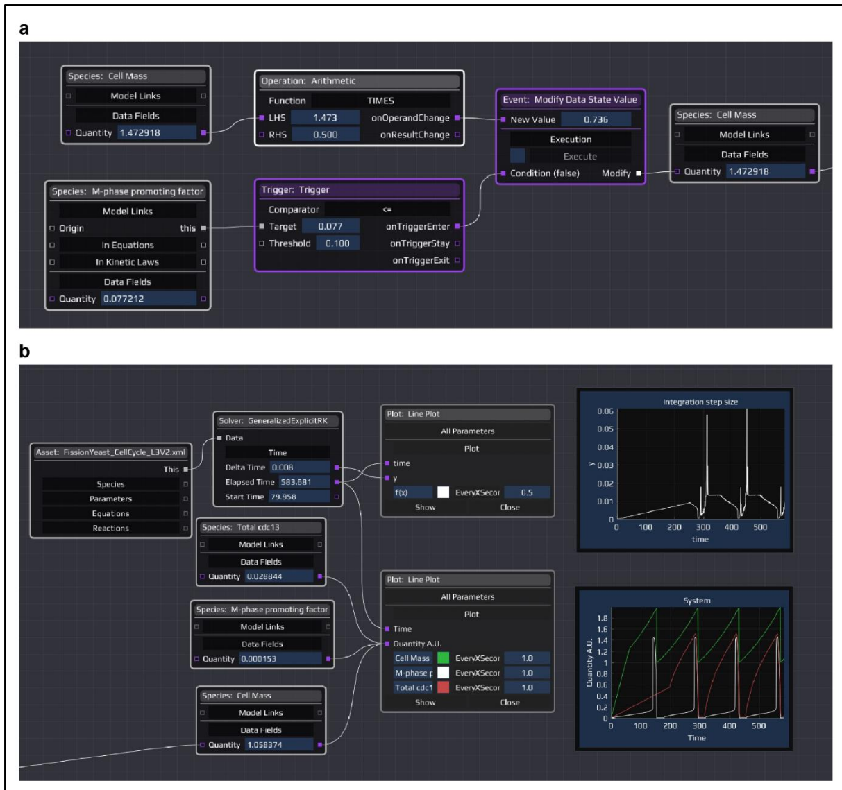
Figure 18: A model of the division cycle of fission yeast (Novak et al., 2001) in ECellEngine. a) Focus on the construction of the event defined in the model using the node-based scripting interface. b) Focus on the visualization of the outputs of the simulation using the node-based scripting interface.
