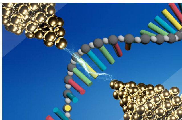
Figure 1.2 Schematic illustration of sequencing for DNA (or RNA) passing through nano-gap electrodes. The colors of each DNA strand represent the four nucleotides, and the color does not signify a specific molecule. As the DNA passes between the nano-gap electrodes, a current is generated by each nucleotide in the DNA. Each nucleotide exhibits distinct electrical characteristics based on its specific chemical structure. Therefore, by analyzing the current over time, DNA/RNA can be sequenced.
