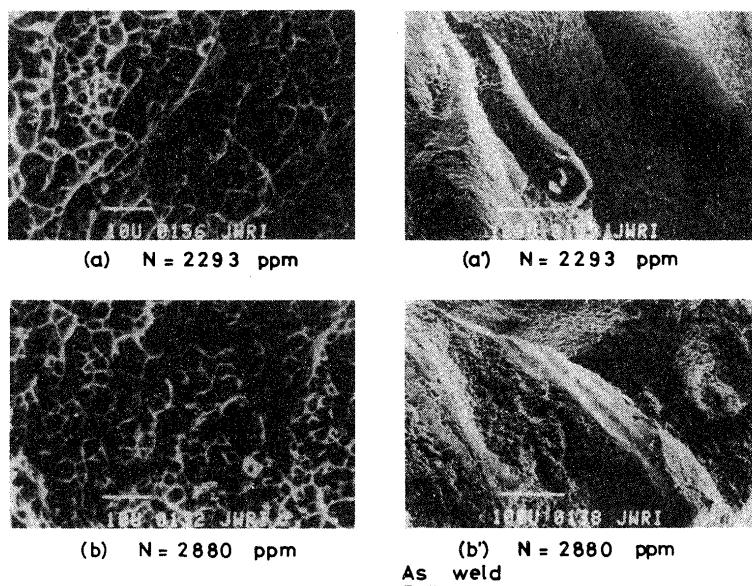
Fig. 9 Change in the fracture morphology of weld metal tested at 77K with nitrogen content. ( $N > 2000$  ppm)
