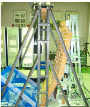
Fig. 15. OOP collapse of specimen CS.
