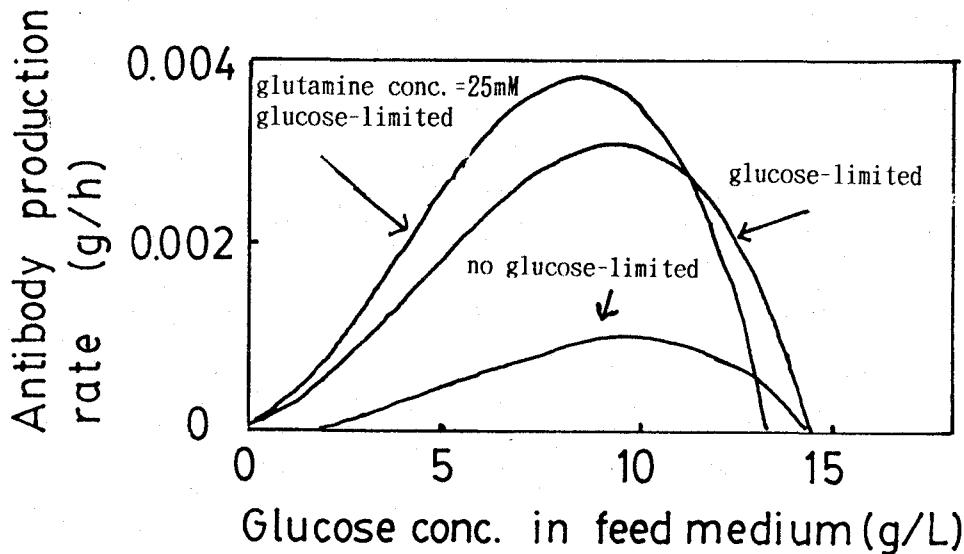
Fig. 5-7 The effect of glucose concentration in feed medium on antibody production rate
