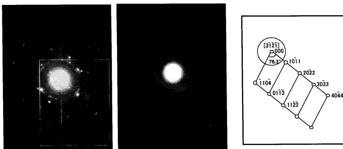
Figs. 2.2. Selected area electron diffraction patterns for (a) the crystalline \text{TiFe}_2\text{N}_{0.53} , (b) amorphous-like \text{TiFe}_2\text{N}_{1.44} , and (c) indexed key diagram for the diffraction pattern shown in (a).
