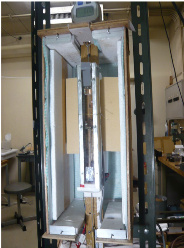
Fig. 1 The thermostated sample space shown with the front panel removed
