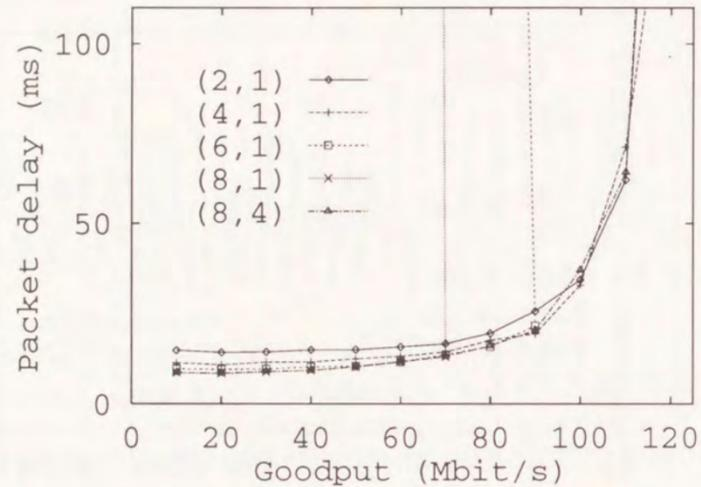
(a). Goodput vs. end-to-end packet delay characteristics.
