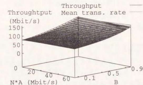
(c). Mean transmission rate and throughput characteristics.
