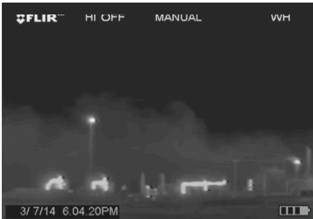
Figure 6. Screenshot of FLIR video of the large release at Marathon Sugarhorn in March 2014. The grey clouds are hydrocarbons (methane and VOCs) rising above the pad site structures, including two flares (the bright white dots) and tanks (Taken by Sharon Wilson)
