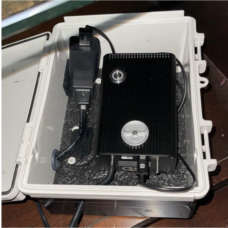
Figure 13. The black carbon monitor, courtesy of Mrs. López
