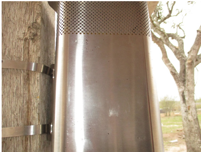
Figure 11. The Omniscent monitor with specks of brown-black solid material hypothesized to be black carbon (Photograph taken by author)
