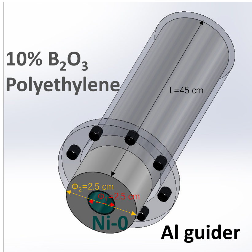
FIGURE 3.11: The structure diagram of neutron collimator used in LDNS experiments.
