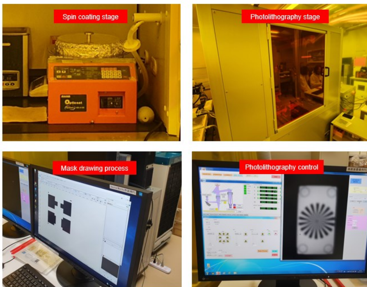
Figure 2.4. Typical lithography setup used in this study
