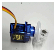
(a) Magnet (right) attached to a servo motor (left blue one)
