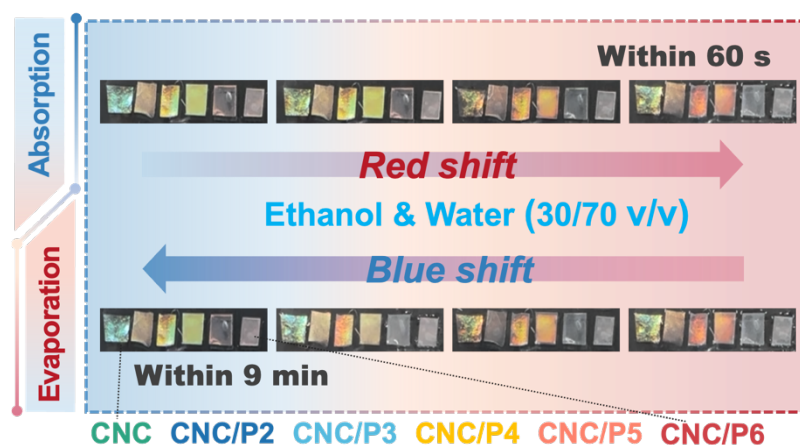
Fig. 3-16. The reversible solvent-responsive process of neat CNC and CNC/PEG-PLA composite films shows the different coloration ranges and response speeds.
