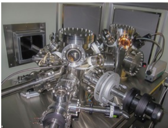
Figure 3.13 Scanning tunneling microscopy equipment.
