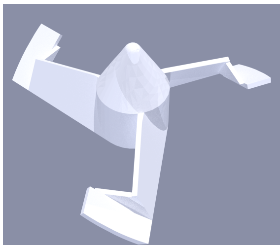
Figure 4.3: Snapshot of the impeller of vertical mixer.
