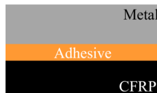
Fig. 1-8 Schematic diagram of adhesive bonding of metal-CFRP.
