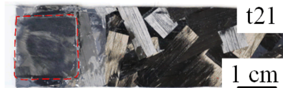
Fig. 2-22 Representative fracture surface of Category 3.
