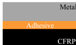
Fig. 1-8 Schematic diagram of adhesive bonding of metal-CFRP.
