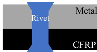
Fig. 1-7 Schematic diagram of mechanical fastening of metal-CFRP.
