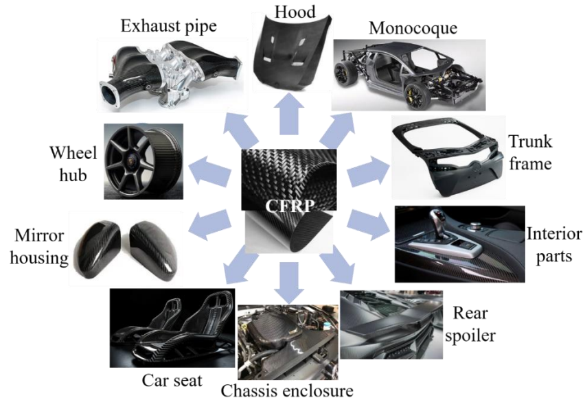
Fig. 1-6 Auto parts made by CFRP.
