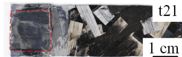
Fig. 2-22 Representative fracture surface of Category 3.
