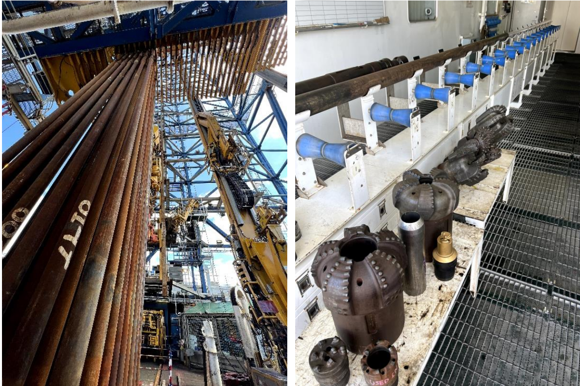
Fig. 1.4 Drill pipes and the drill bits in the Chikyuu vessel
