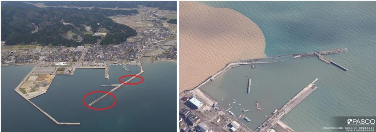
Figure 1.4. Aerial view of Iida Port before (left) and after (right) the damage to the eastern breakwater. Red circles indicate the position of the loss of the east breakwater (Sato T., 2024).
