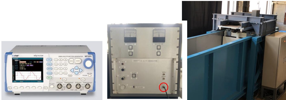
Figure 5.4. Multifunction Generator WF1973/WF1974 (left), operation panel of wave generator (center) and piston-board station at one end of the wave flume (right).
