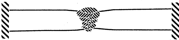
(b) Type 2 distortion that involves Mode 1 and Mode 2 movements caused by free surfaces being joined before the solidification of the weld metal
