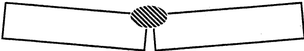
(c) Type 3 distortion caused by Modes 1 and 2 movements and Mode 3 rigid body movements
