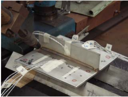
Fig.3 Experimental set up of fillet welding
